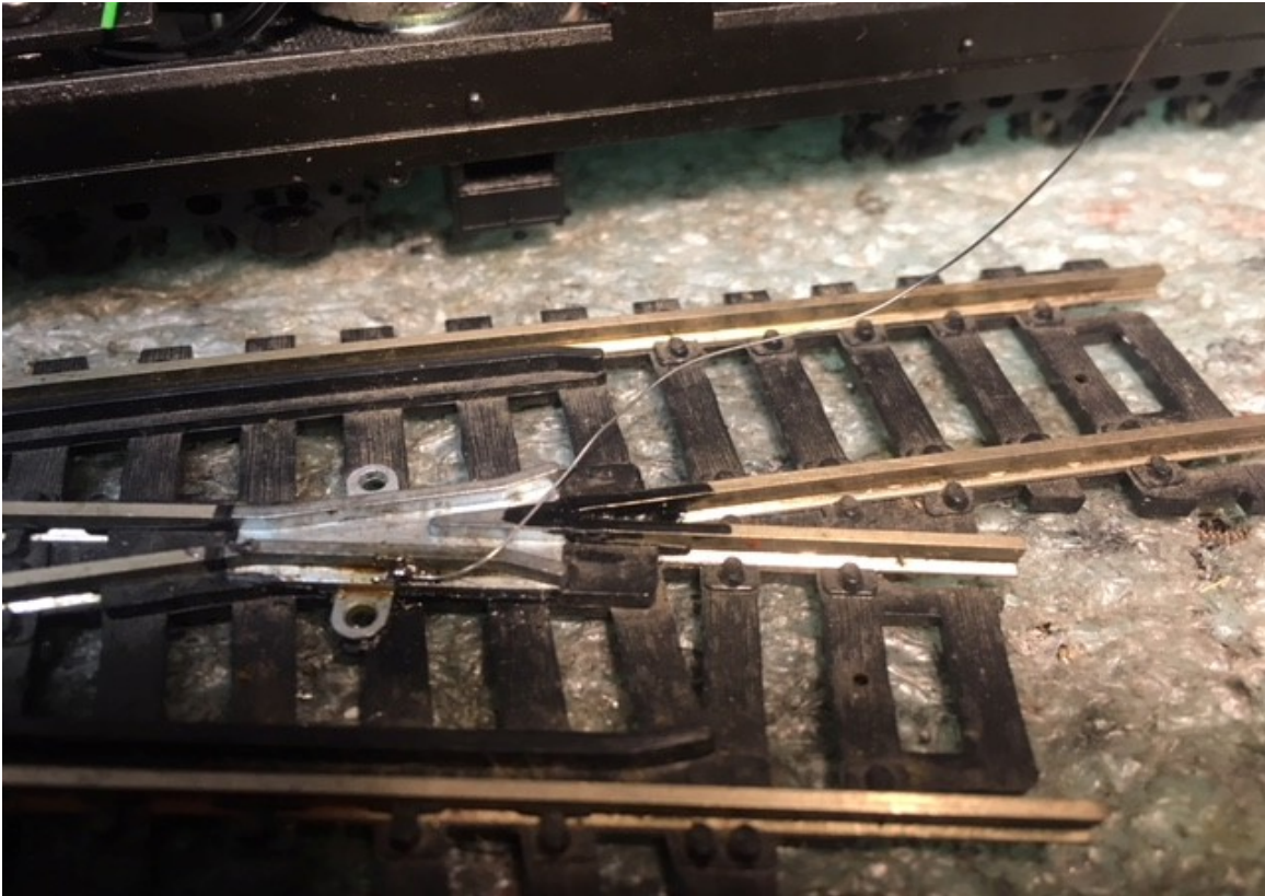
Illustration 2: 30 Gauge wire soldered to Atlas Zinc die-cast frog
