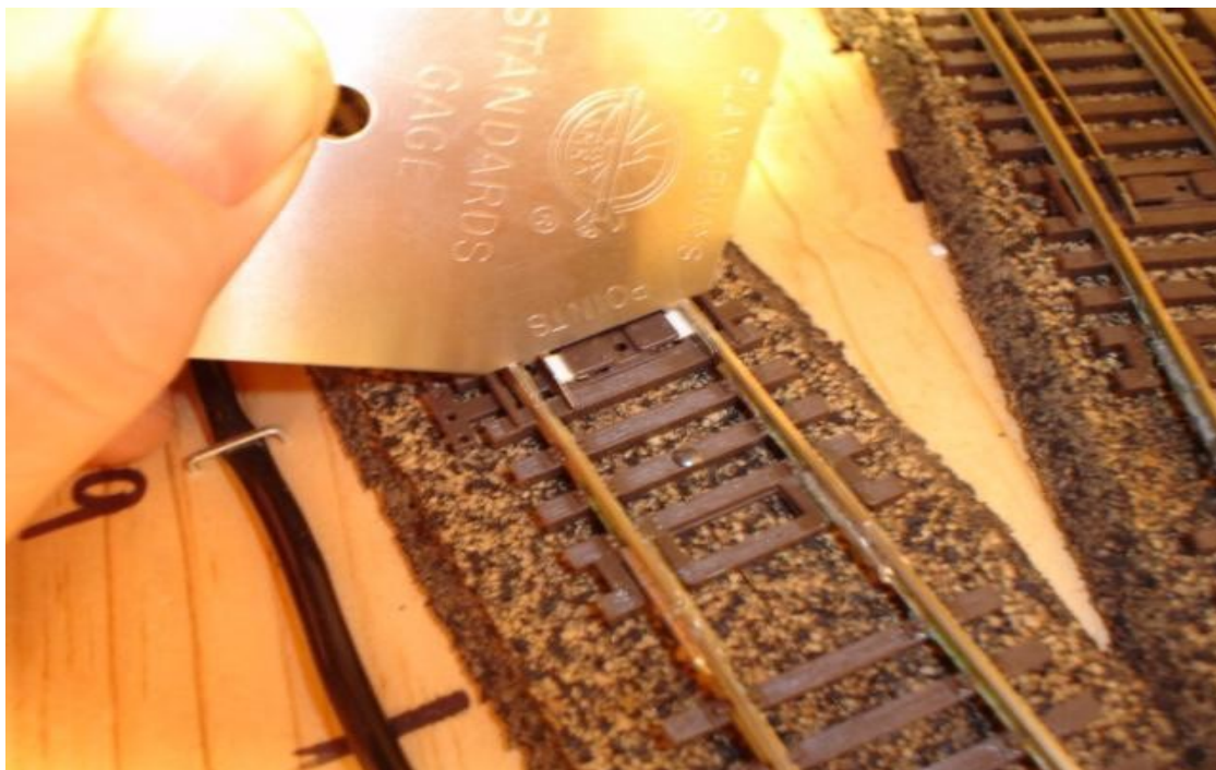
Illustration 25: The NMRA gauge makes the improvement apparent
