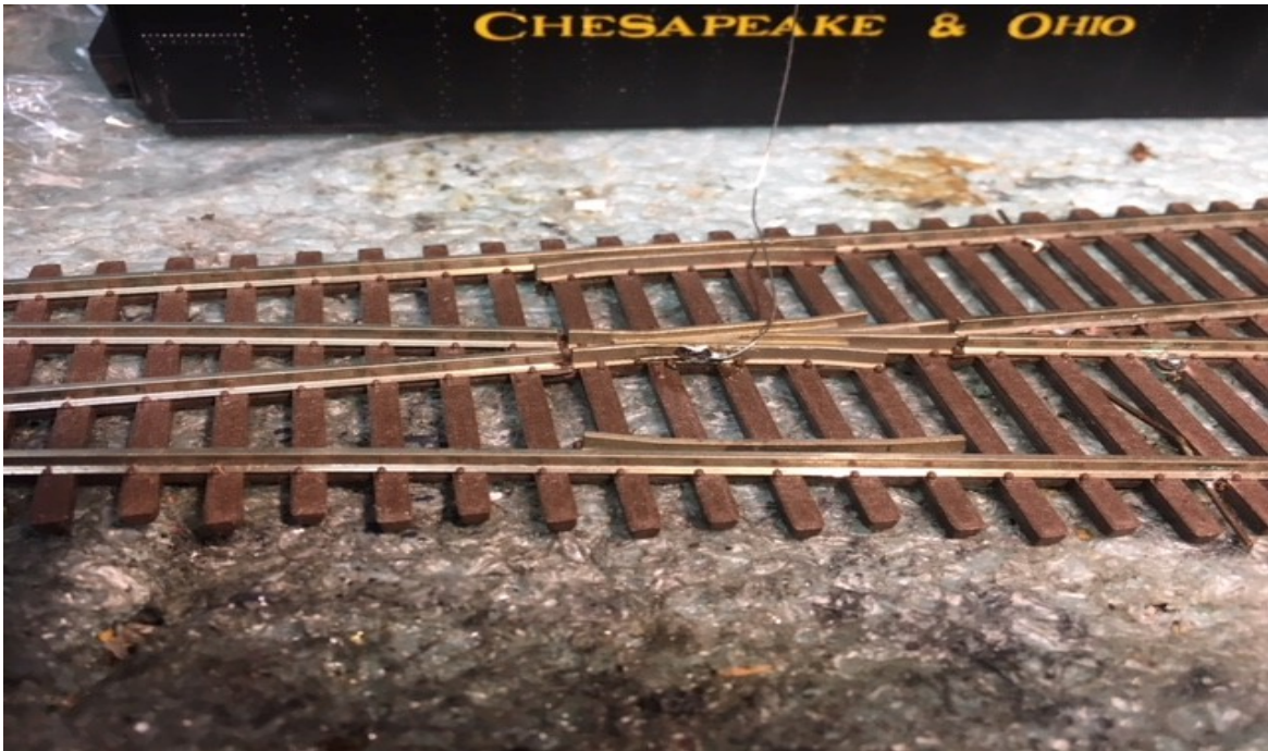
Illustration 3: Solder Connection to Micro-Engineering Frog Web
