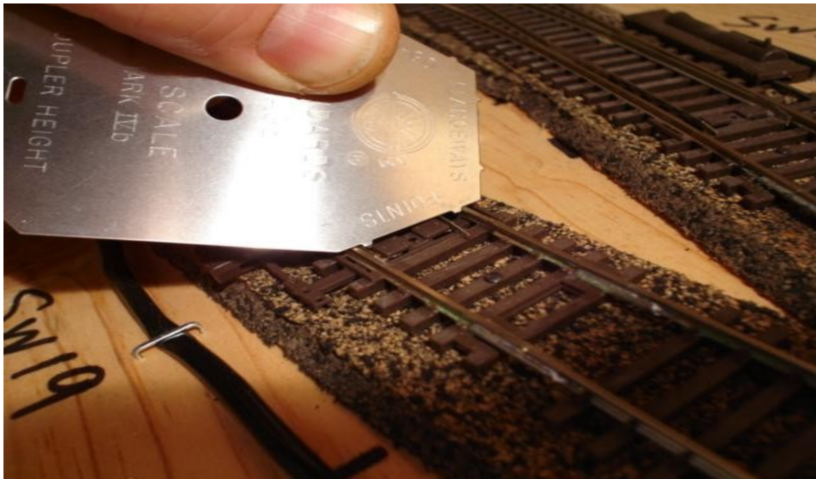
Illustration 23: Same as above-with NMRA gauge inserted
