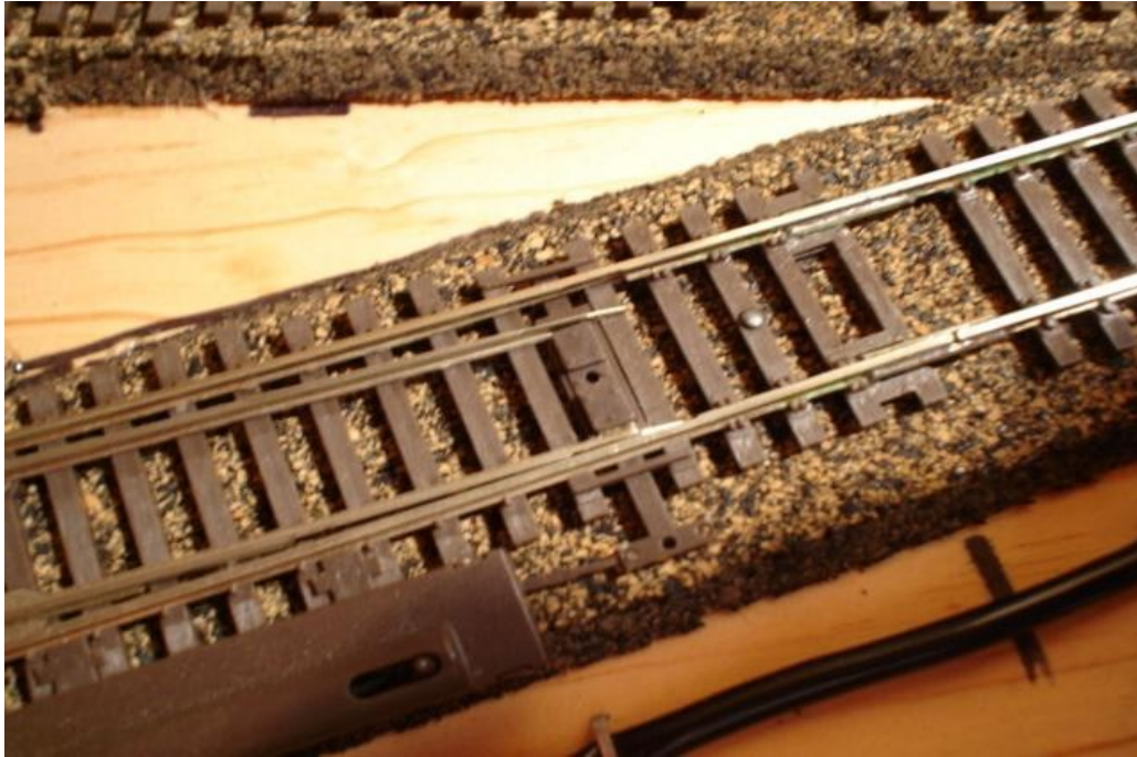
Illustration 22: Atlas point rails - out of gauge (too narrow)
